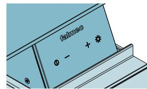
To access the push-button panel, the top panel must be opened: this activates the motor at speed 1.
